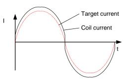
Coil current does not have optimum shape
